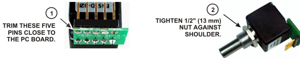
Figure 13. Checking and Trimming the VFO B Encoder Pins.
